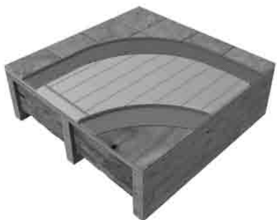
WarmWire over wood frame floor with backer board
