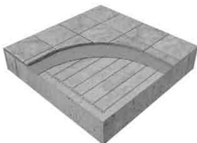
WarmWire over concrete slab.
