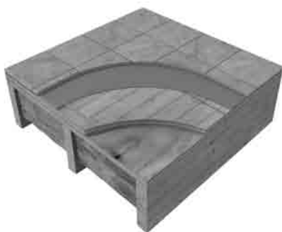
WarmWire over wood frame floor with double plywood
